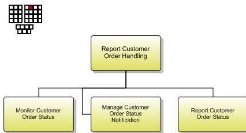
Figure 4.10 Report Customer Order Handling decomposition into level 4 processes
